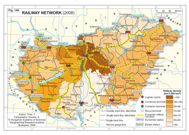
are constituents of the European corridors; the majority of logistic centres, combined and container terminals, and RoLa terminals are located alongside them. Rebuilding the international main lines so that they are suitable for speeds of 120–160 km/h and the installation of modern signalling systems are under way with EU assistance. However, on 60–70% of the branch lines, passenger trains can only travel at 20–35 km/h because of the obsolete technology.
