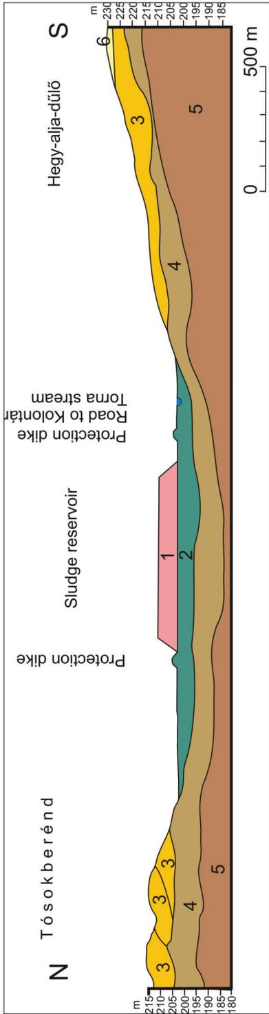
Fig. 3. Spoil heaps and sludge reservoirs upon the alluvium of Torna stream between Ajka and Tósokberénd (ed. by JUHÁSZ, Á. 2003). – 1 = sludge reservoir, spoil heap; 2 = alluvial sequence (sand, gravel, silt); 3 = terrace built of alluvium (gravel, sand) of the ancient streams (Torna, Csigere); 4 = Somló Formation (Pannonian sand, clay); 5 = slope loess, sandy loess, clastic gravel sequences
